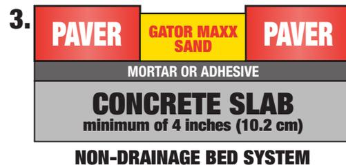
For diagram 3, the pavers are adhered to the concrete slab using either a thin set mortar or a permanent bond adhesive.
